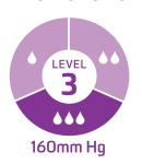
BFE (%): ≥ 98 PFE (%): ≥ 98  $\triangle$  P (mmH<sub>2</sub>0/cm<sup>2</sup>): <6.0 Fluid Resistance: 160mm Hg Flame Spread: Class 1
