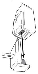
2. Slide the wall plug or line cord onto the transformer until it is firmly seated.
